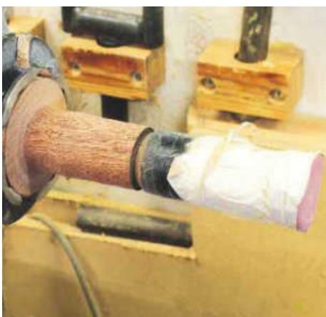
STEP 26. The bark edge dictates that I can't drive the piece off the top. This stem that locates in the bottom will allow me to mount the work up. A piece of abrasive on the end will prevent it from marking the inside
